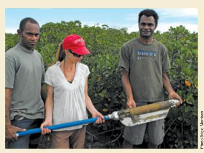
Figure 38. Russian peat corer at Fiji core site LW3.
