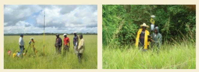
Figure 22. The RTK system, composed of (a) setting a base station by static surveying (left), and (b) RTK mode with both base (left) and rover (right) working together (Kimeu & Machano, 2011).
