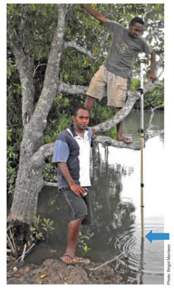
Figure 27. Reference station (h) at Lomawai, Fiji. The survey stake is vertical, secure at its base and taped to the tree branch for the survey period. The arrow shows the water depth to record at the same time depths are recorded in the mangroves.
