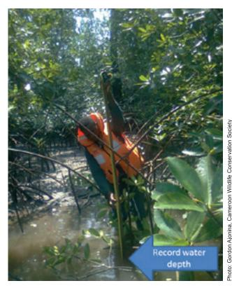
Figure 28. Recording water depth at sample sites (d) within the mangroves at the same time as a measurement is taken at the reference station (h).
