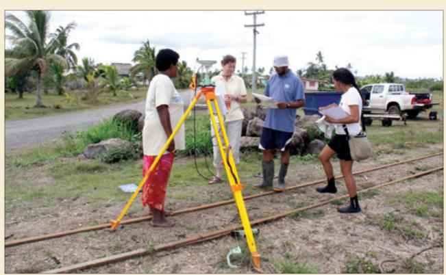
Figure 30. Surveying a temporary benchmark to datum using differential GPS, Lomawai, Fiji.
