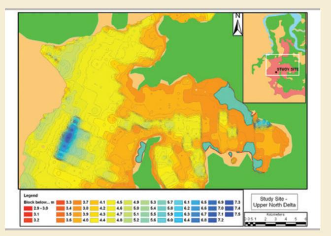
Figure 24. Raw elevation results from differential GPS survey of the central section of the North Rufiji Delta inland mangrove study area (Kimeu & Machano, 2011).
