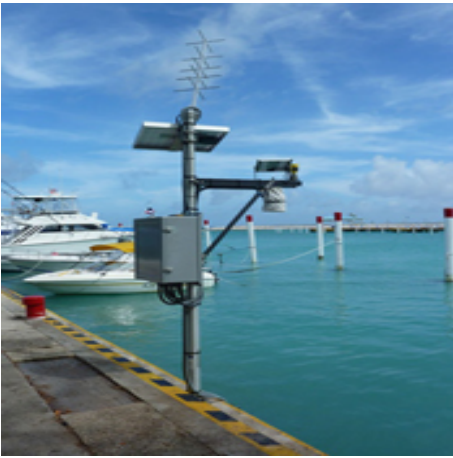
Figure 1. Tide gauge station (credit: NOAA Climate Observation Program)
