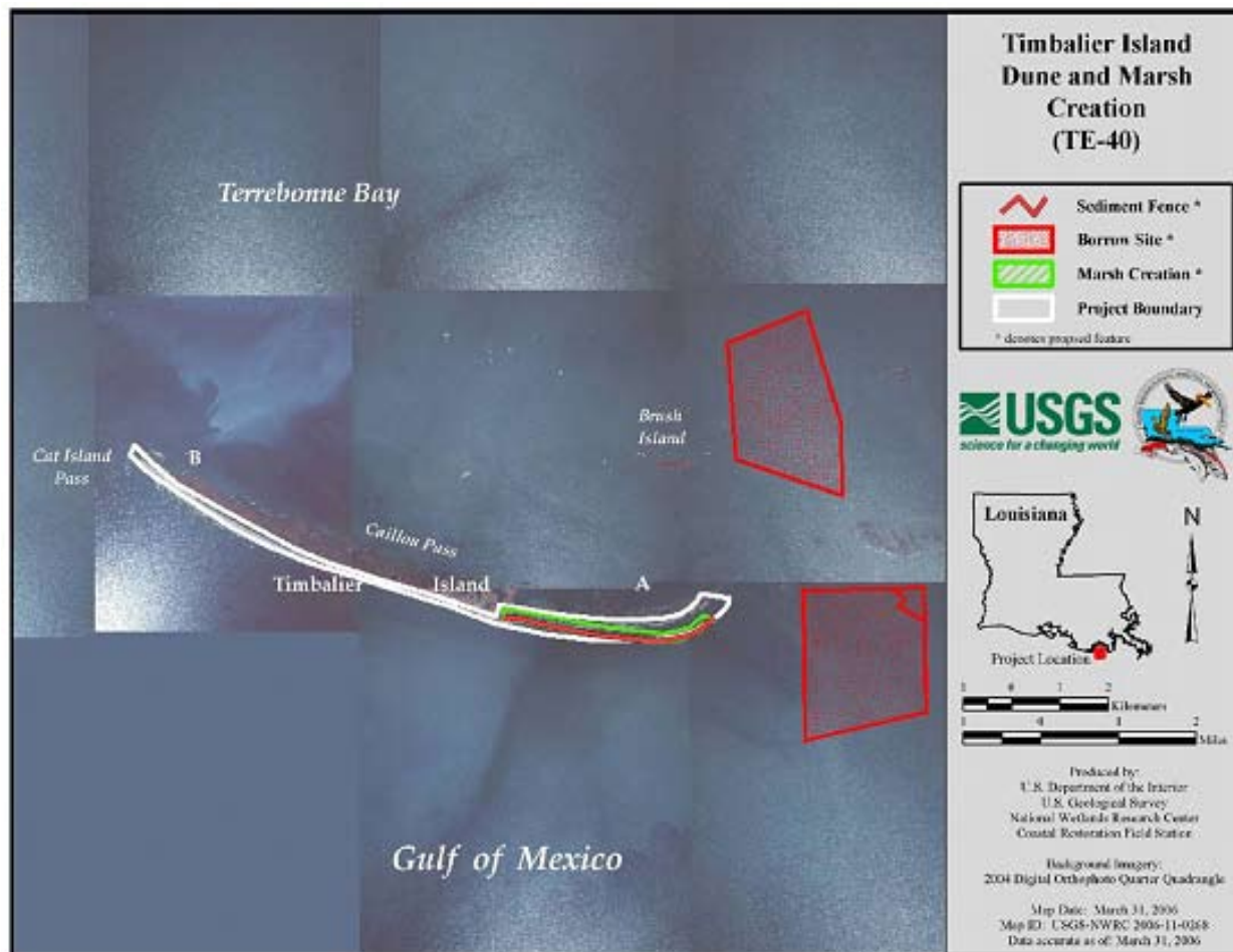
Figure 3.2-4. Map of Timbalier Island with the placement areas for the dune and marsh shown in green and yellow and the borrow areas in Little Pass Timbalier to the east of the island shown in red.
