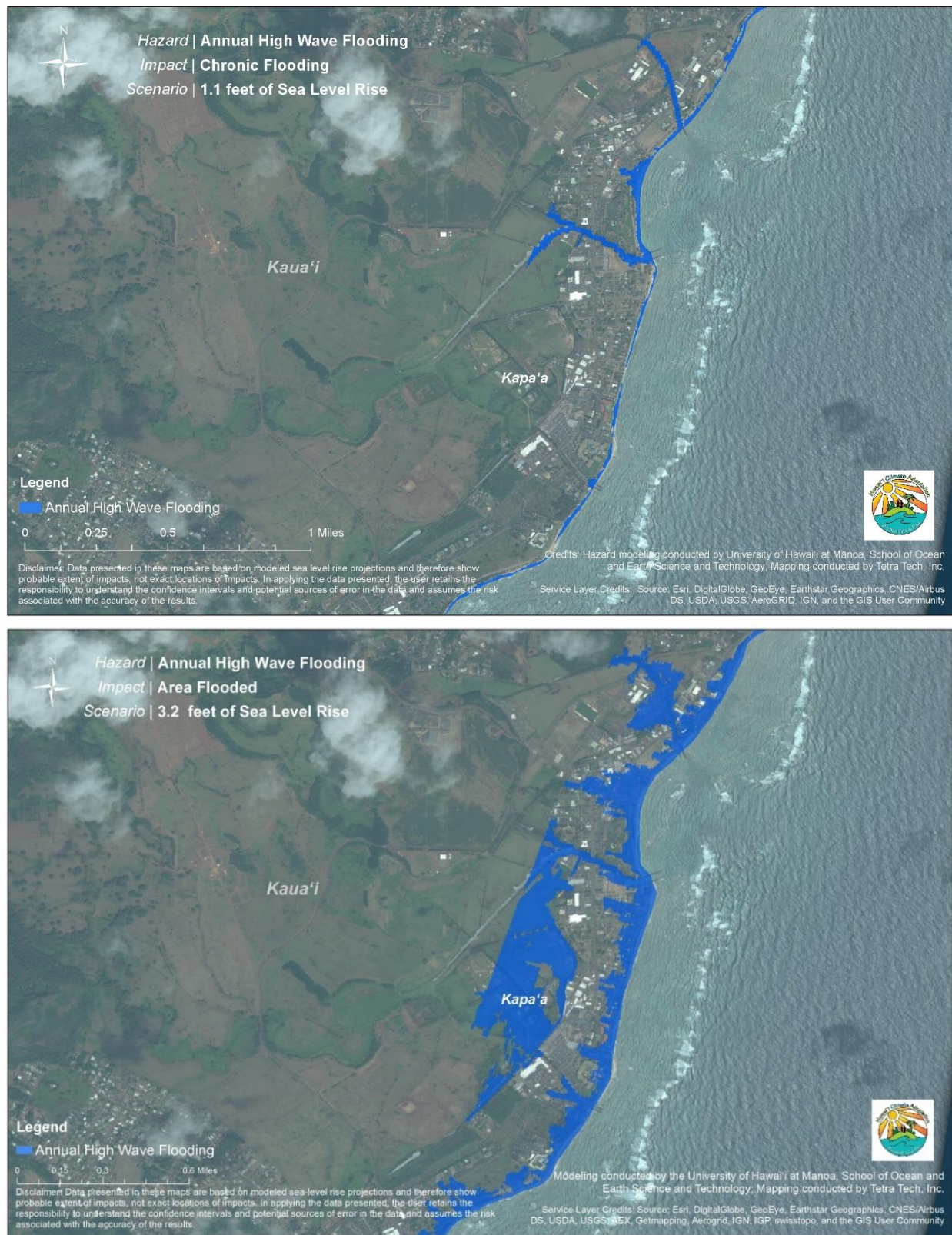
Figure 25. Example maps showing results of annual high wave flood modeling with 1.1 feet (top) and 3.2 feet (bottom) of sea level rise for Kapa'a, Kaua'i
