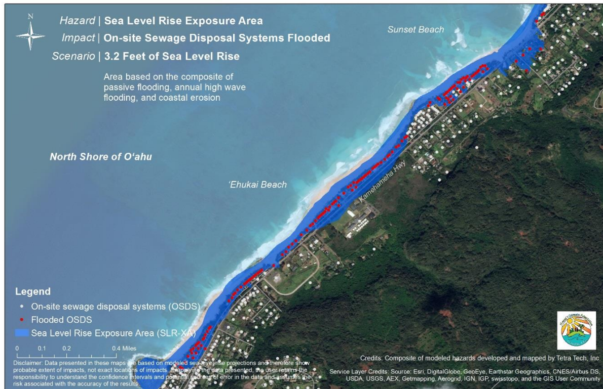
Figure 110. On-site sewage disposal systems flooded in the SLR-XA with 3.2 feet of sea level rise along the North Shore of O'ahu
