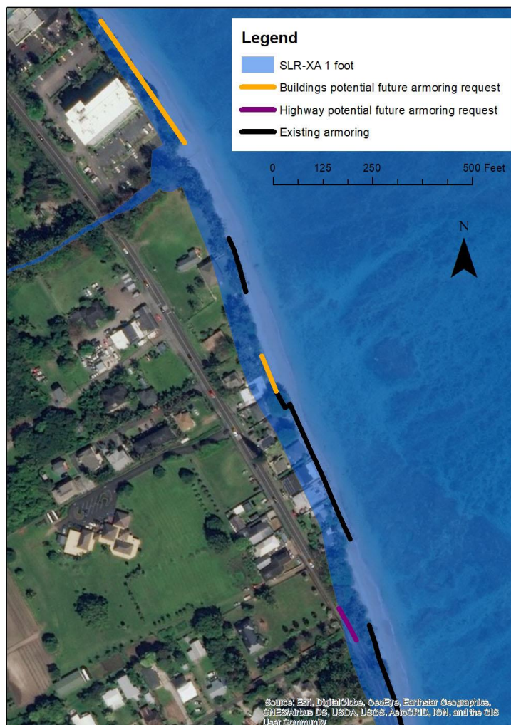
Figure 34. Example map of existing shoreline hardening (black) and potential future shoreline hardening and beach loss based on the SLR-XA with 1 foot of sea level rise for exposed beachfront properties (orange) and coastal roads (purple) for a section of Punalu'u, O'ahu
