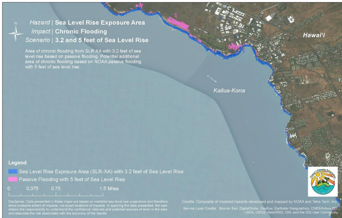
Figure 52. Potential additional area of chronic flooding with 5 feet of sea level rise in Kailua-Kona on the Island of Hawai'i
