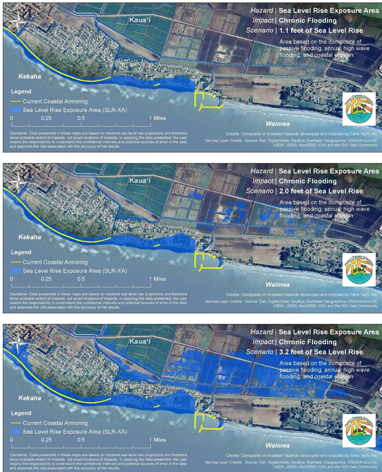
Figure 114. Potential chronic flooding in the SLR-XA with 1.1, 2.0, and 3.2 feet of sea level rise in Kekaha, Kaua'i
