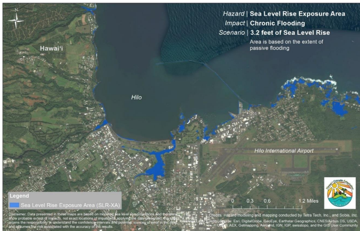
Figure 45. Key transportation facility, Hilo Harbor, in the SLR-XA with 3.2 feet of sea level rise on the Island of Hawai'i
