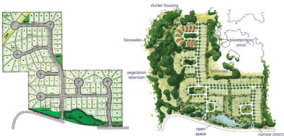
Figure 3.12: Conventional site design (left) with an LID-based design (right).
