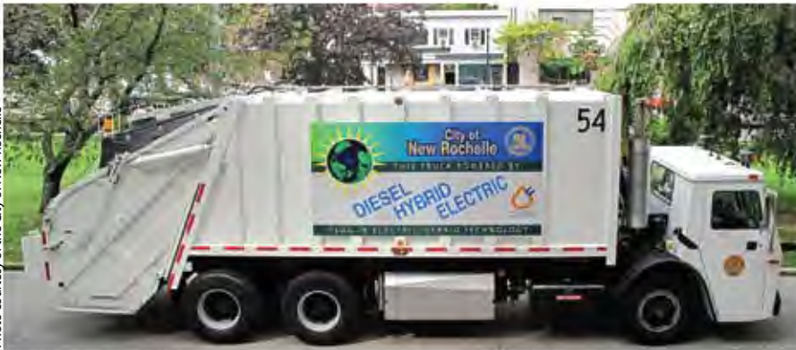
Syracuse's not-for-profit 'Cuse Cars program rents out low-emission cars for short-term use, which helps the city move toward carbon neutral transportation. New Rochelle's diesel hybrid electric garbage truck also helps in reaching a carbon-neutral future by costing less for fuel and emitting less greenhouse gas.
