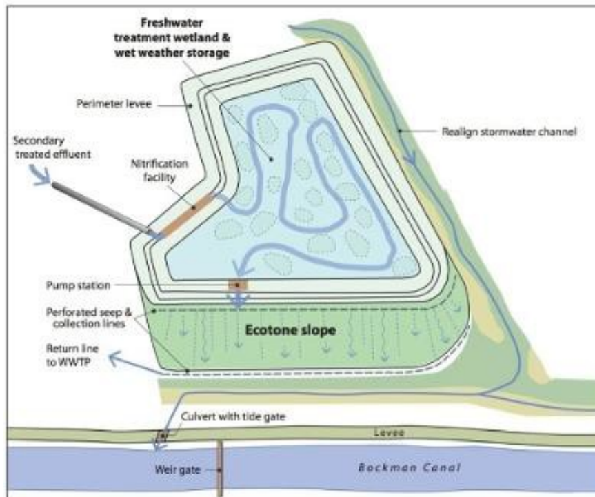
Figure 1: Plan view of the wet weather treatment basin and horizontal levee/ecotone slope (ESA).
