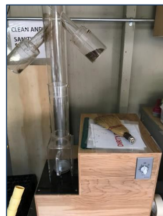
Figure 7. Seed cleaning machine used for Oro Loma project.
